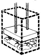
When operating, the compacting ram does not go all the way to the drawer bottom. You will not see compacting of the first few loadings.
